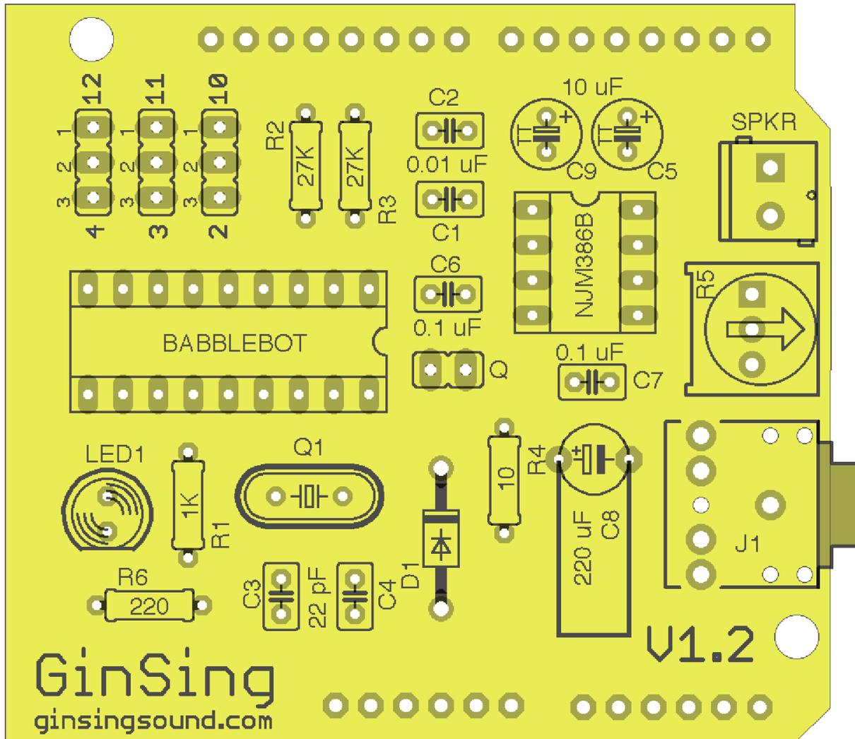
Take a minute to examine the circuit board. You will notice that the each part and its corresponding value are marked on the silkscreen.
