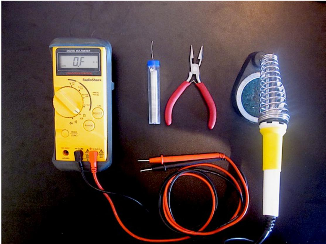
The GinSing hardware requires only a couple of tools and basic soldering skills. You will need to have a good working **soldering iron**, **solder**, and **side cutter** | **needle nose pliers** If you are just starting out we highly recommend this [beginners toolkit](#).
